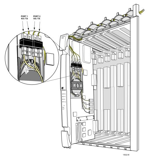
Figure 701-7. Fiber Connectors on an 155 SM/MM CRS Card
